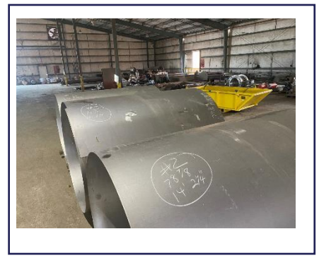
Figure 17: Preparation of the new liner.
