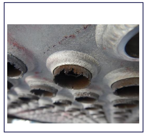
Figure 11: Severe crosscut end attack.
