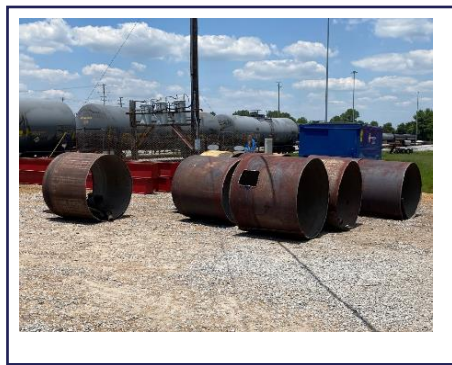
Figure 16: Removed Zirconium liner.
