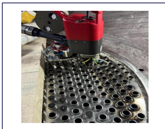
Figure 13: Orbital welding of the top tube sheet
