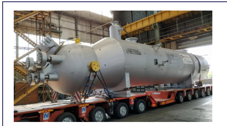
Figure 21: Kettle-type HPCC in proprietary E-type steel.
