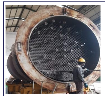
Figure 24: Grid design HP stripper.
